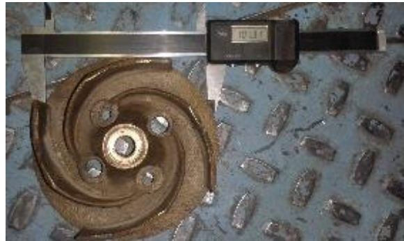
Figure 3: View of the pump's impeller
